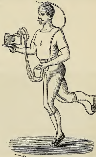
FIG. 195.—Marey's apparatus for recording movement in locomotion.
